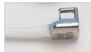
Fig. 2: 1.5PSL Probe for mouse ascending aorta blood flow.
