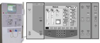
The Override key is used for two functions. One is to override a blood leak alarm for three minutes and keep
