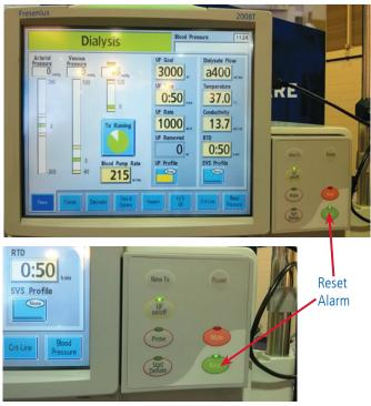
Press and Hold the Reset Button for two seconds to spread the arterial and venous pressure alarm limits by 300 mm Hg and fully open the TMP pressure for 30 seconds. This can be performed as the saline line is opened to allow the infusion of saline. Thirty seconds should be enough time to prevent an Arterial or Pressure alarm. If more time is need the Reset can be pressed and held again to allow for another 30 second alarm speed.
