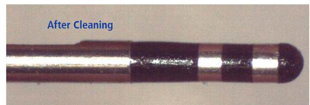
**1.2F Rodent Pressure Volume Catheter before (top images) and after (bottom images) proper cleaning. A 30 min wash in 1% Tergezime (Alconox Inc.) removes the dried liquid and blood. See Catheter Cleaning and Disinfecting Guide (CDS 2.06) for complete instructions.**
