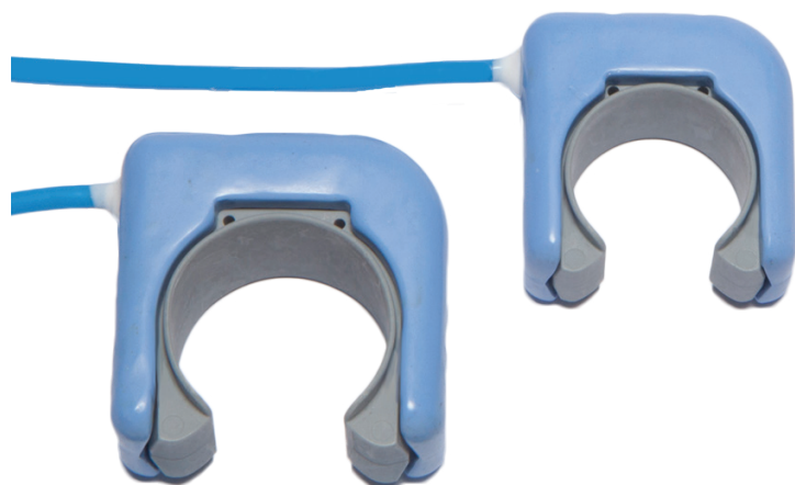
Fig. 6: Two CONfidence Flowprobes® fitted with Ultrafit liners.
