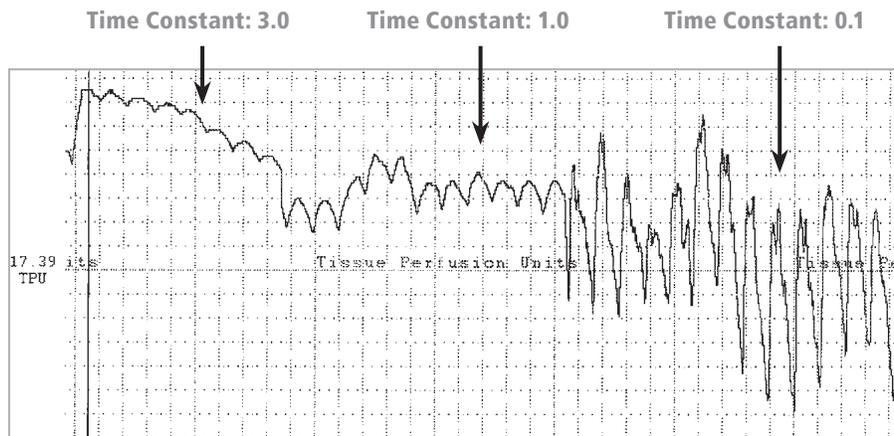
Fig. 1: Index finger blood flow using Type R Probe first with time constant switch on 3.0, then 1.0 and finally 0.1 sec.
