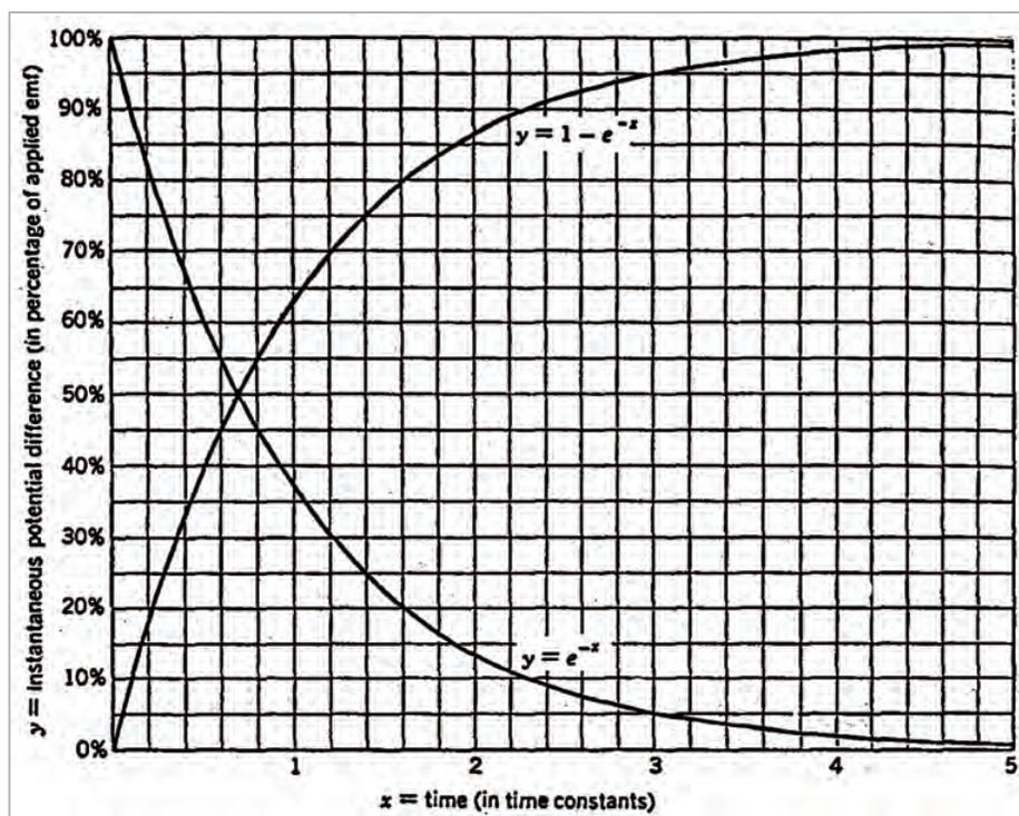
Fig. 3: Universal exponential curves for the graphical solution of the charge and discharge of capacitors in DC circuits<sup>1</sup>.
