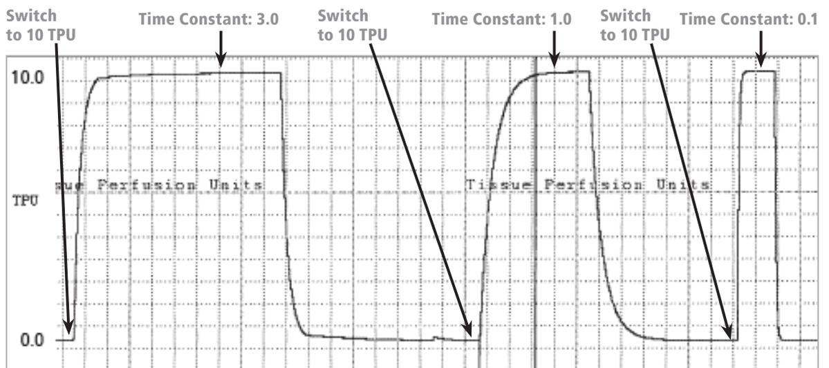
Fig. 2: Recorded by switching to calibration mode (10 TPU), allowing the output to maximize and then switching the mode back to "0" then allowing the signal to fall, for each of the three time constants. This shows the effect of time constant setting on signal output. Note the time required for the signal to reach full scale.
