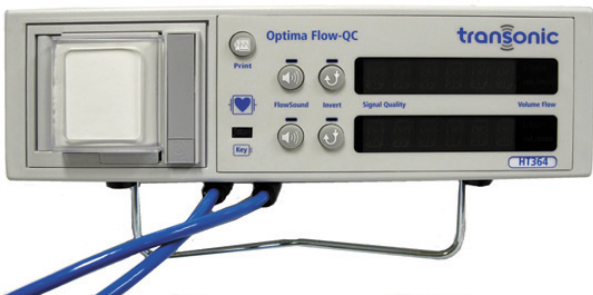
HT364 Optima dual-channel Flowmeter for simultaneously measurements of aortic and pulmonary artery flows.
