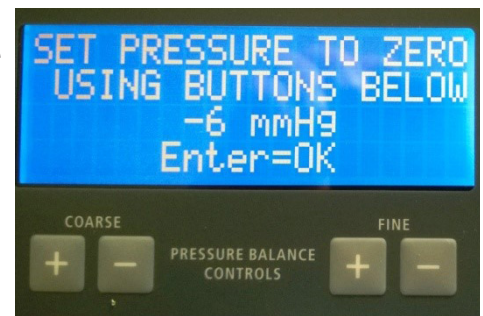
Adjust Pressure #2 menu. Use the buttons below the screen to adjust the zero offset
