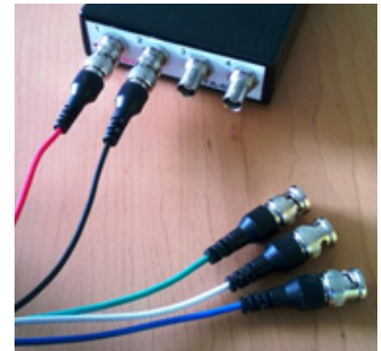
The red BNC output is for pressure sensor 1 and the black is for pressure sensor 2. All other outputs should not be connected.
