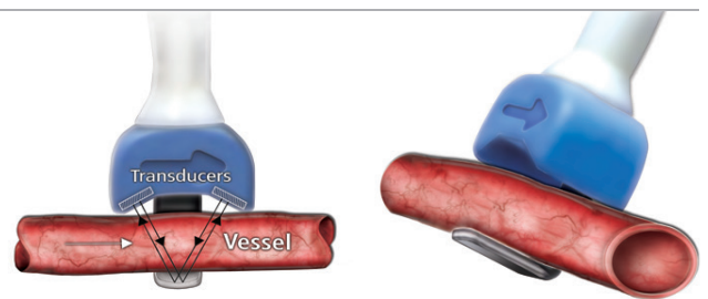
Fig. 1: Transonic® non-constrictive perivascular volume flowprobes use wide beam illumination as two transducers pass ultrasonic signals back and forth, alternately intersecting the flow in upstream and downstream directions. By deriving an accurate measure of the "transit time" it takes for the ultrasound waves to travel from one transducer to the other and calculating the difference between the integrated transit times, volume flow, not velocity is measured.
