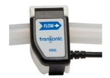
Transit-time ultrasound technology measures volume flow in tubing with specifically designed Tubing Flowsensors. Most non-aerated liquids can be measured, including saline and buffer solutions, blood and water. No physical contact is made with the fluid media. H-XL Series Flowsensors can be calibrated and programmed for up to four different fluid/temperature/tubing combinations and will work with most flexible tubing types (see next page). Sensor size is determined by outer tubing diameter.
