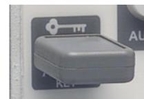
Selected HT300-Series Flowmeters (HT314, HT354, HT364) are activated by inserting a disposable Flow-QC Key. If the meter is turned on without a Flow-QC Key, the Flowmeter displays [INSERT KEY].
