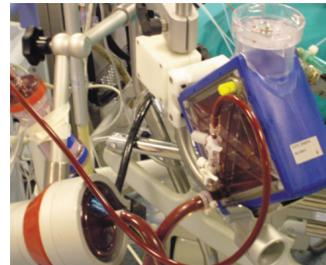
Shown is a Maquet Quadrox oxygenator in use. It is by far the most common type of ECMO oxygenator. Whatever the model, oxygenators all share the same tendency to clot. During a case, it is impossible to see through the flowing blood to identify the underlying amount of clot that has formed. Physicians and perfusionists are not taught about variance in clot formation and clots can differ.
