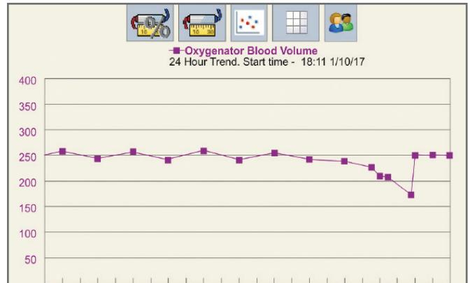
Each injection is plotted. Here you can see where the volume decreased (as clot volume increased), and returns to baseline when the oxygenator is changed out.
