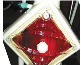
Non-flaking soft clots evenly spread across the fibers shown here cause a high pressure gradient. This would tempt some teams to change out the oxygenator, even though it is still functioning well. That would not be a good move, as changing an oxygenator is risky (zero flow for a couple of minutes, and potential air embolism) as well as detrimental loss of RBCs, clotting factors, proteins, etc., in the oxygenator.
