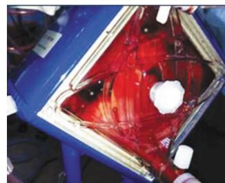
Shown in this oxygenator is a thin, soft layer of clot over most of the fibers with some fibers exposed so there is no pressure gradient change. Mixed density, some hard formations growing.
