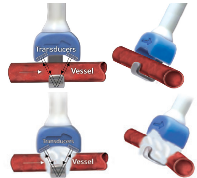
Fig. 1: Upper graphic shows a Perivascular Flowprobe without acoustic couplant. Bottom graphic shows the same Flowprobe with acoustic couplant filling the spaces between the Probe and the vessel.
