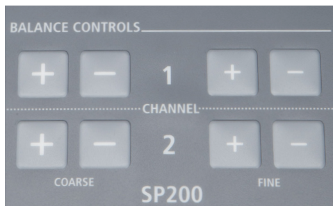
Fig 5. Channel 1 pressure balance controls on SP200 are on top. Channel 2 pressure balance controls are on the bottom.
