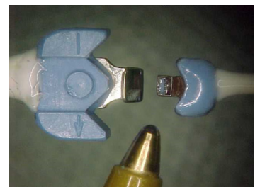
Fig. 2: V-Series and PS-Series probes next to a ballpoint pen tip for scale.
