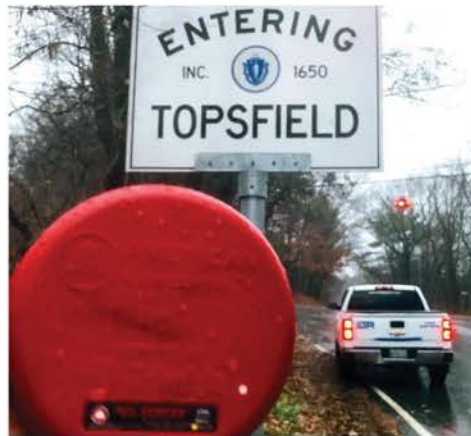
AFC SEMPER RPMs used to identify system pressure issues.
