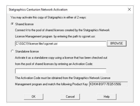
Set the radio button to "Shared license". Using the *Browse* button, locate the file *sgcnet.usr* in the license directory which was created in Step 5. Then press *OK*. This should launch the program and display the main window:
