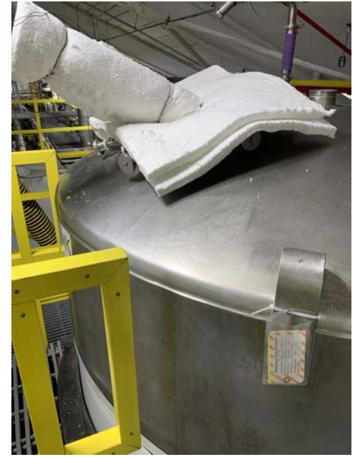
(Above Left) The heat curing equipment is set up to cure the ChemLINE® coating to spec. (Above Middle) The vent is set up to move the fumes out of the manufacturing facility. (Above Right) Heat cure equipment with an insulated vent extended from the heat curing equipment into the tank. (Bottom Right) Fully cured topcoat layer inside the storage tank.
