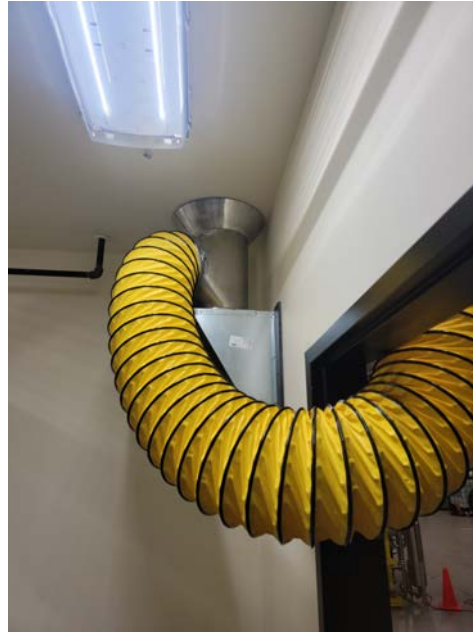
(Above Left) The heat curing equipment is set up to cure the ChemLINE® coating to spec. (Above Middle) The vent is set up to move the fumes out of the manufacturing facility. (Above Right) Heat cure equipment with an insulated vent extended from the heat curing equipment into the tank. (Bottom Right) Fully cured topcoat layer inside the storage tank.
