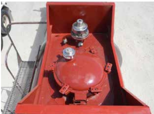
(Above) Manway lid showing corroded rubber lining, due to HCl exposure. (Below) Manway lid and surrounding spill area properly protected with ChemLine® coating.
