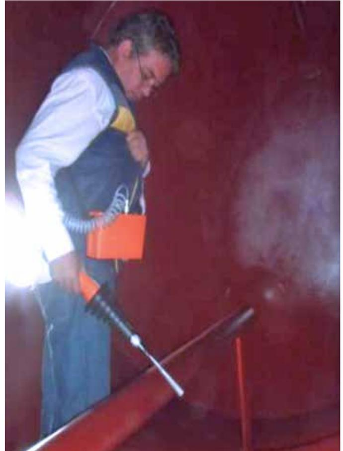
*This Sulphuric Acid storage tank at Monómeros Colombo Venezolanos uses ChemLine® 784/32 coating for superior corrosion protection. Here, prior to being put into service, the coating in the tank is spark tested as part of a thorough inspection process.*
