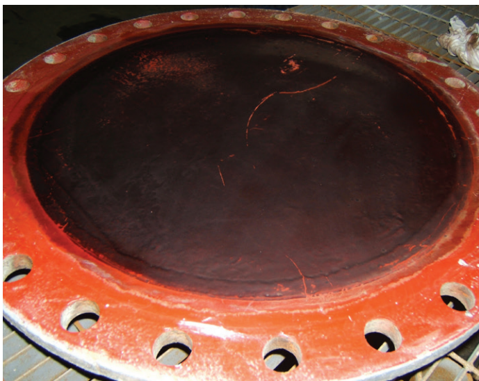
ChemLine® 784/32 coating intact after 10 years service (left). Staining can be removed (right).
