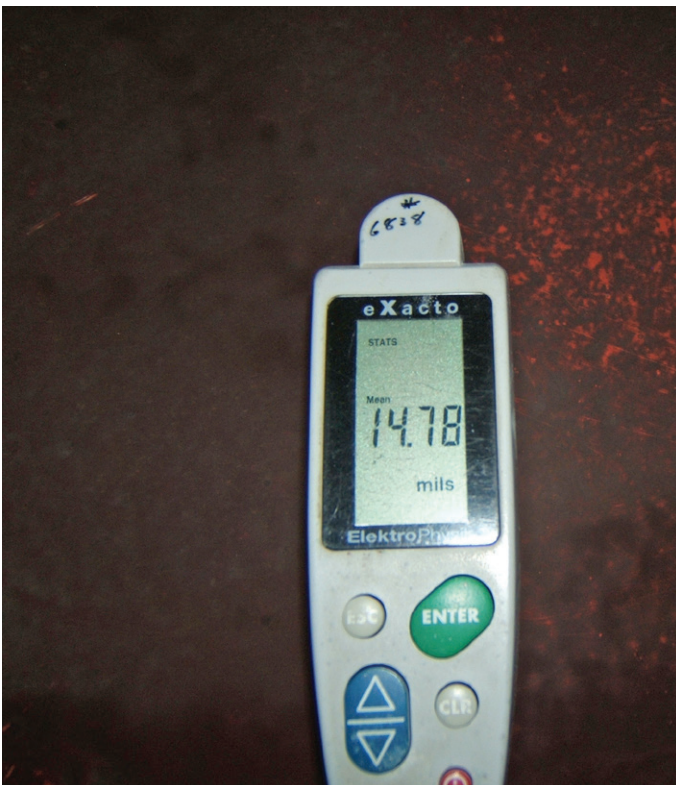
Staining from acid (left). No loss of coating thickness (right).
