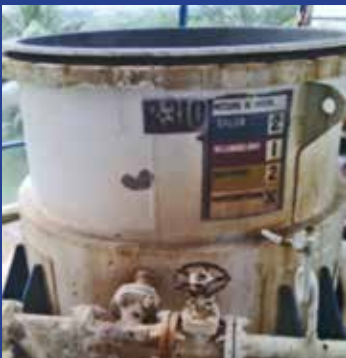
(Left) The R-310 reactor vessel. (Center) Reactor first lined and protected with ChemLine® in 1998. (Right) Reactor vessel in 2001 before re-coating.
