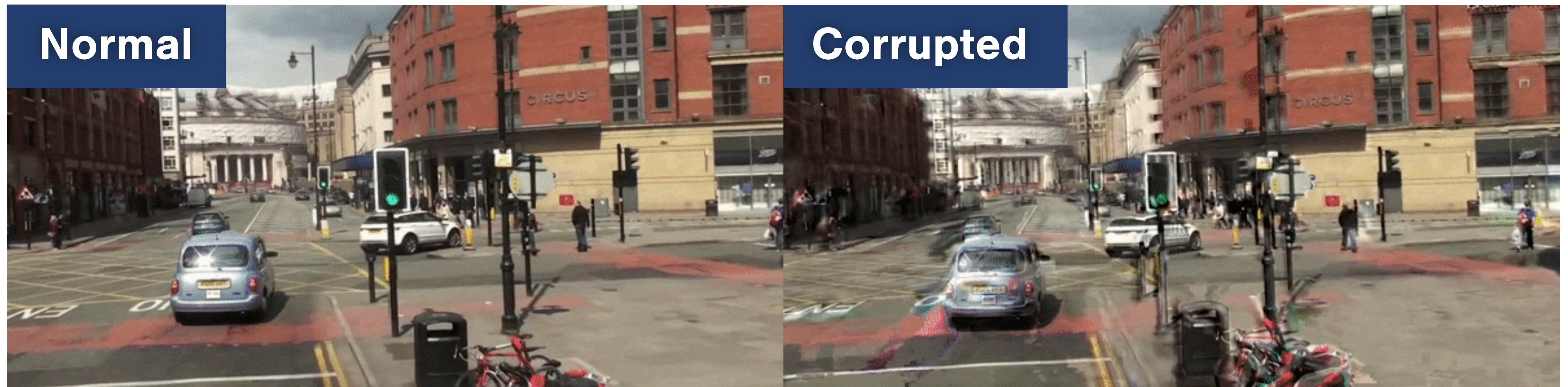
Normal video on the left side, visible P-frame corruption on the right side. Observe color and shape irregularities, increased posterization.
