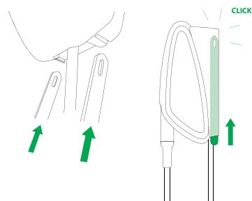
Now you can remove your charging station from the wall dock. Pull the charging station away from the wall dock in a straight line.
