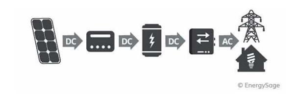
Example of DC-coupled system: DC electricity flows from solar panels to a charge controller and feeds it directly into a battery. An inverter is used to transform DC into appliance-friendly AC. Any electricity produced will be inverted once, flowing from your batteries to your home or out to the grid.
