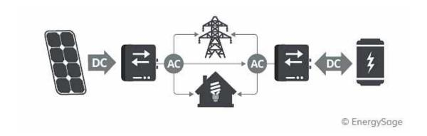
Example of AC-coupled system: DC electricity flows from solar panels to an inverter that transforms the energy to appliance-friendly AC. To store it in a battery for later use, it will need to flow through another inverter, transforming it back into DC.
