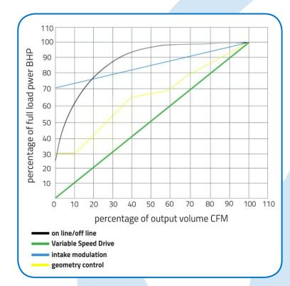
PneuTech's variable speed drive technology combined with a direct drive, permanent magnet motor reduces energy and maintence costs up to 50%
