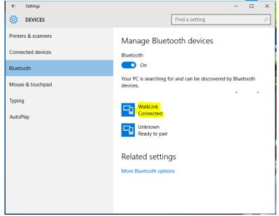
Find the COM port associated with that connection. Go back to WALKLINK CONFIGURATION WIZARD/ALTERNATE METHOD, select the matching COM port and SAVE the configuration. Device Manager/Ports(COM & LPT) shows the COM port number. Ensure you have the WalkLink showing blinking blue light and WalkAnalyst WalkLink indicator light is lit.
