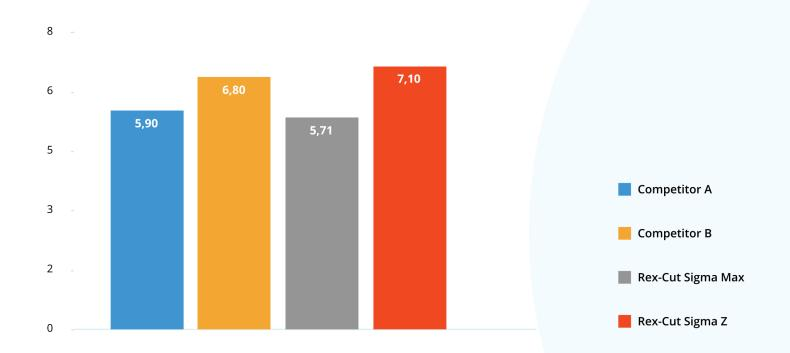
Sigma Z on average removes 7.1 inches of 304 Stainless Steel per minute.
