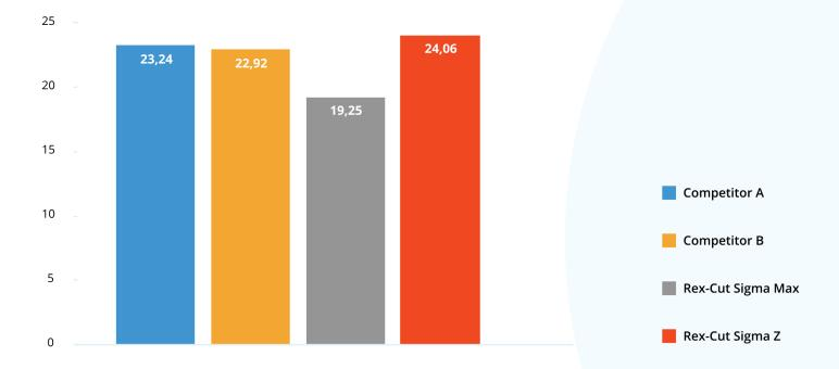
Sigma Z removes an average of 24.06 grams of 304 Stainless Steel per minute.
