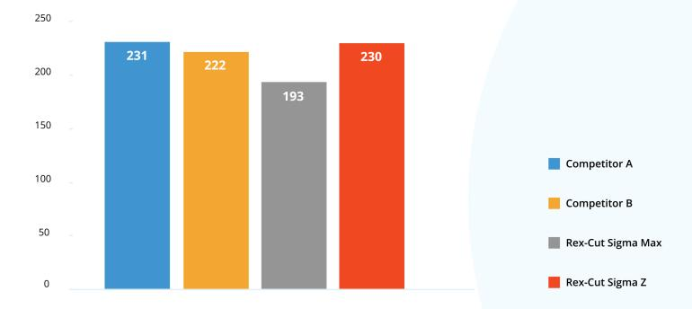
Sigma Z leaves a Surface Roughness of 230 on 304 Stainless Steel.
