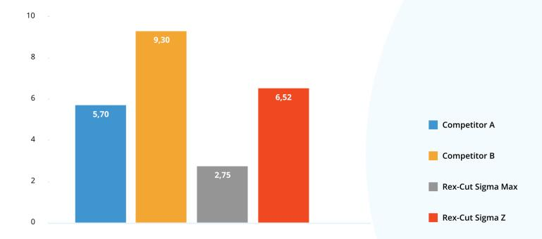
Sigma Z Grinds on average removes 6.52 grams of 304 Stainless Steel per 1 gram of wheel loss.
