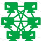
The N366 is deployed as a mesh node, with the built-in self-backhaul connecting to additional N366 devices, TUs, or to a network POP. The POP connection can be via ether fiber or our EtherHaul™ PtP links with up to 10Gbps full-duplex capacity. The ability to create multiple self-backhaul links enables diverse traffic routing to support differentiated SLA levels, as well as carrier-grade make-before-break redundancy with sub-50ms traffic switch-over.
