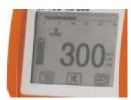
An important feature of the Variotec 460 tracer gas is that it contains 2 sensors. The low level sensor is used to measure very small levels of gas, parts per million (ppm), and the second sensor automatically measures the higher levels of gas, Vol %.
