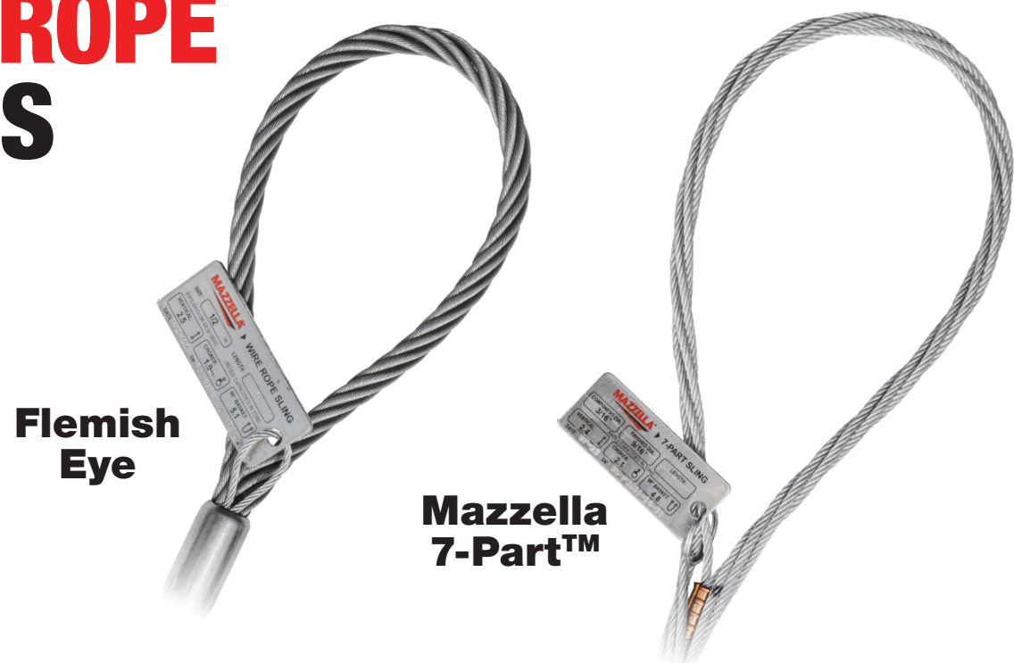
Flemish Eye Wire Rope Slings IWRC EIP Flemish Mechanical Spliced (6 x 19, 6 x 36 Class)
