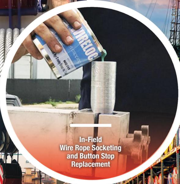
**In-Field Wire Rope Socketing and Button Stop Replacement**
