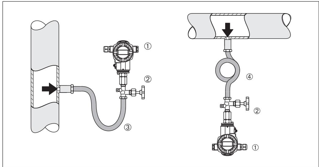
Fig. 7: Measuring arrangement for pressure measurement in steams
