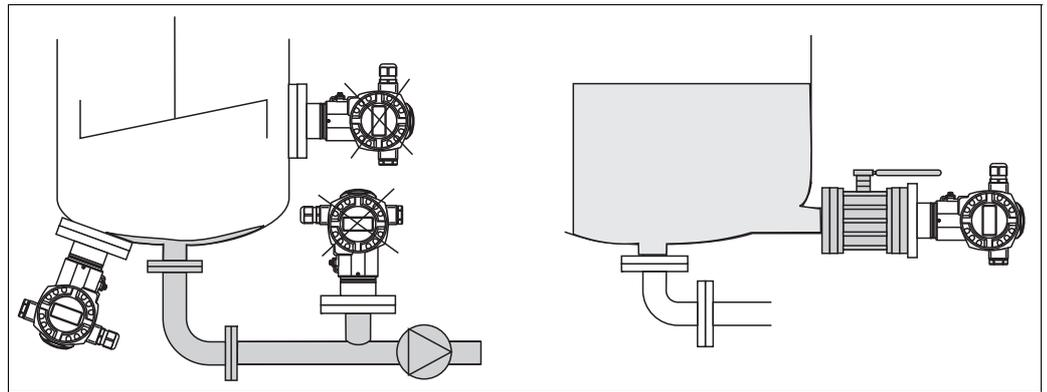
Fig. 9: Measuring arrangement for level
