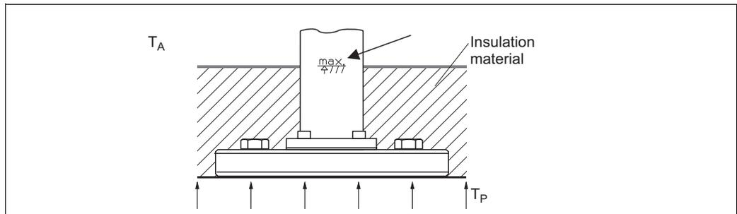
Fig. 14: Maximum insulation height, here e.g. PMC71 with flange
