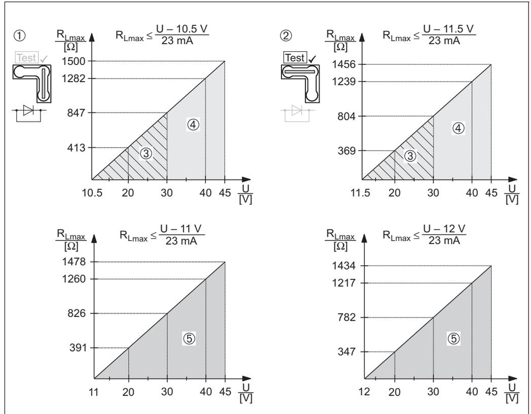
Fig. 21: Load diagram, observe the position of the jumper and the explosion protection. (→ § 28, "Taking 4 to 20 mA test signal" part.)
