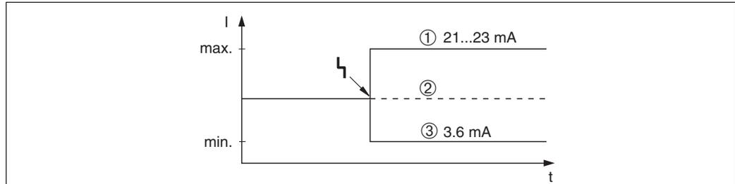
Fig. 26: Current output in the event of an alarm
