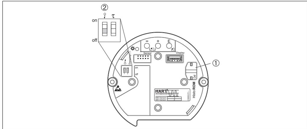
Abb. 24: Electronic insert with optional HistoROM®/M-DAT memory module
