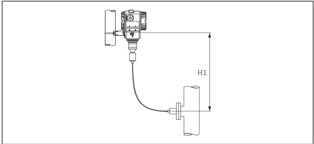
Fig. 10: Installation above the lower diaphragm seal
