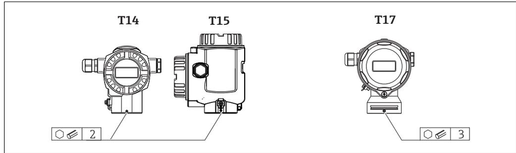
1. T14 and T15 housing: Loosen setscrew with a 2 mm (0.08 in) Allen key.
