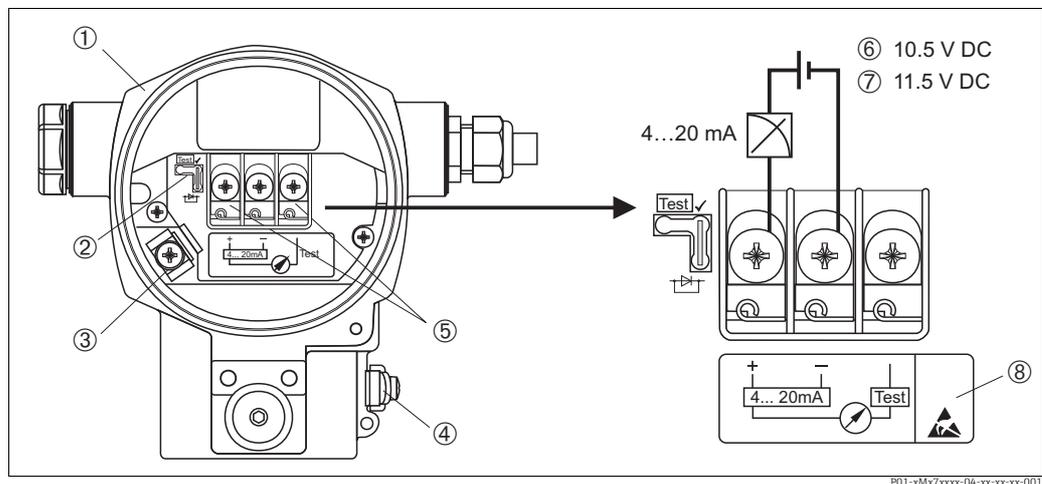
Fig. 18: Electrical connection 4 to 20 mA HART. Observe also → 28, "Supply voltage".
