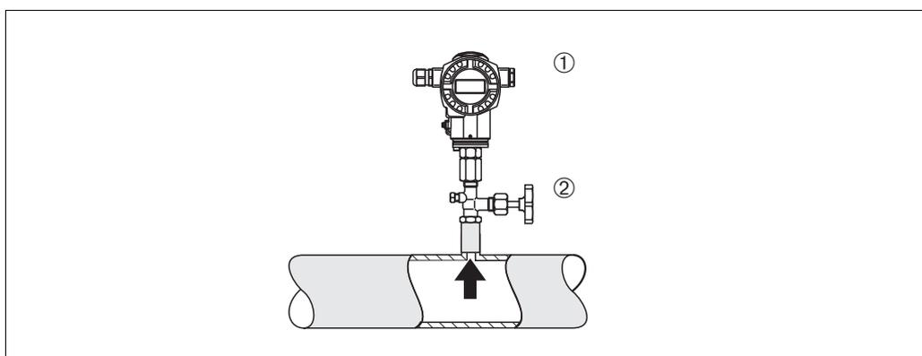
Fig. 6: Measuring arrangement for pressure measurement in gases
