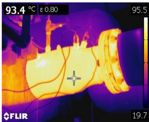
Figure 13 This thermographic image is of a large bore pipe and flange to the boiler.
