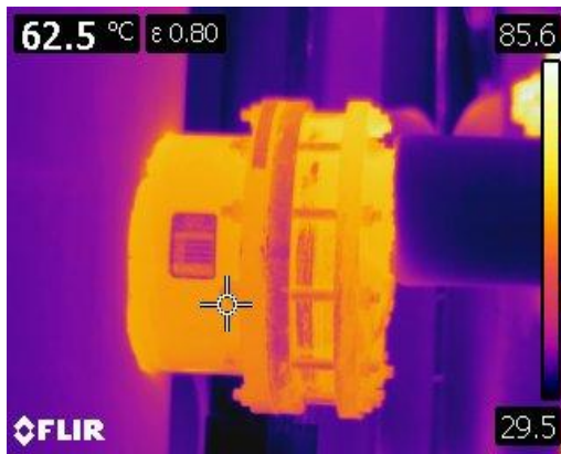
Figure 31 Thermographic image of heat exchangers in the hot water tanks.
