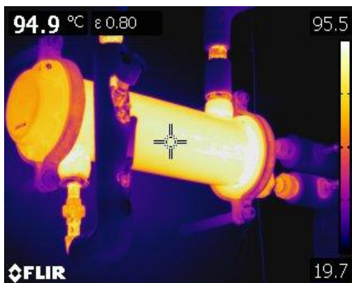
Figure 17 Thermographic image of a wall mounted heat exchanger that is a source of heat loss.
