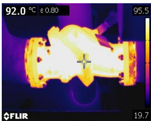
Figure 19 Thermographic image of a control valve overhead in boiler room.
