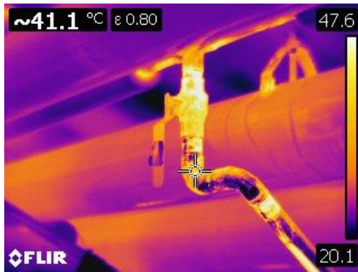
Figure 41 Thermographic image of bare copper heating line in penthouse fan room.
