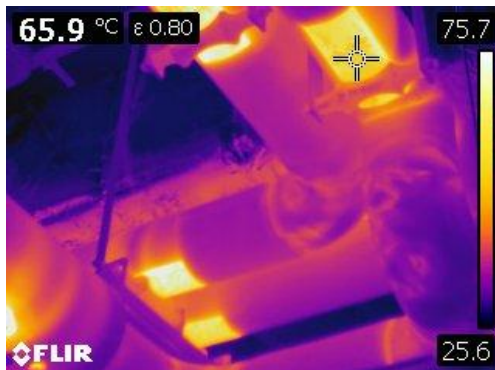
Figure 39 Thermographic image of the pipe supports that have no insulation behind them. There are over 60 of these.
