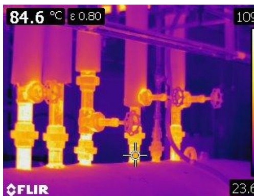
Figure 17 Thermographic image of valves and unions on top of a vessel at 84° C or 183° F
