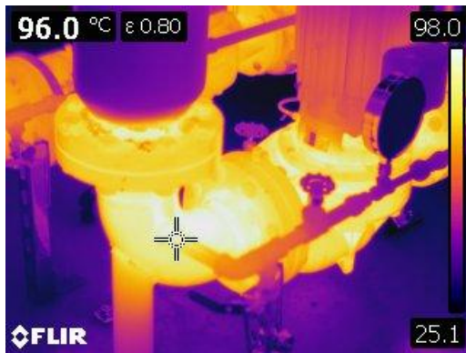
Figure 31 Thermographic image of heating supply pumps at 101° C or 213° F.
