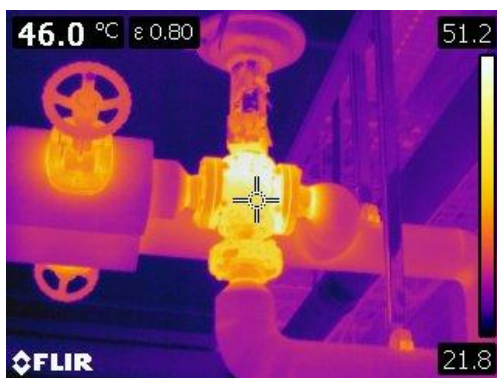
Figure 57 Thermographic image of bare three way valve and bare bonnets at 46° C or 114° F
