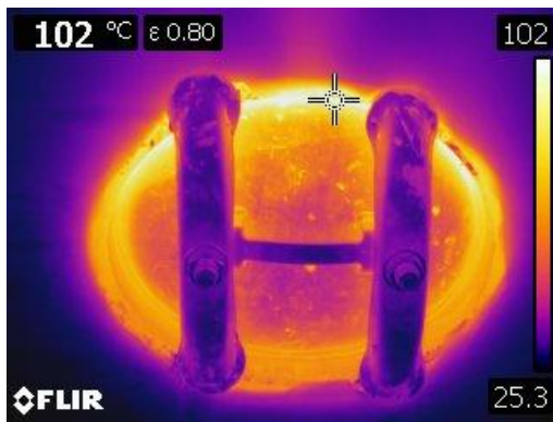
Figure 19 Thermographic image of the access hatch to this vessel at 102° C or 215° F
