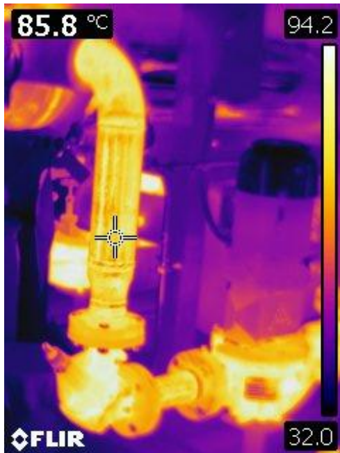
Figure 65 Thermographic image of bare motorized heating pump and piping at 85° C or 185° F
