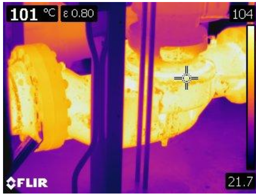
Figure 31 Thermographic image of heating supply pumps at 101° C or 213° F.
