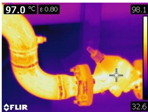
Figure 67 Thermographic image of bare pipe and control valve and motorized pipe at 97° C or 206° F
