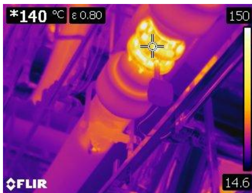
Figure 21 Thermographic image of a flow meter at 140° C or 284° F.
