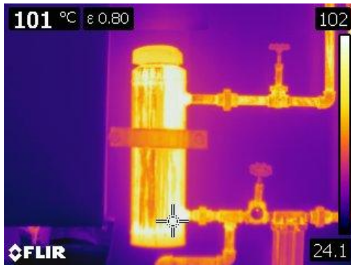
Figure 37 Thermographic image of a chem. pot at 101° C or 213° F.
