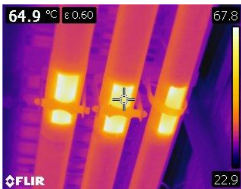
Figure 49 Thermographic image of bare three way valve and bare valve bonnet at 86° C or 186° F
