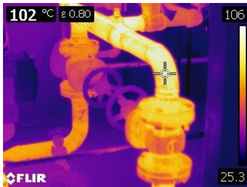
Figure 13 Thermographic image of one specific valve bonnet but the image shows many bare areas missing insulation.
