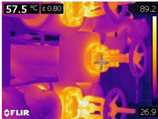
Figure 69 Thermographic image of bare valve bonnets at 57° C or 134° F
