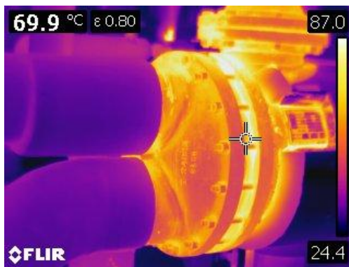
Figure 59 Thermographic image of bare heat exchanger head at 69° C or 156° F
