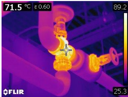
Figure 53 Thermographic image of large three way valve and bare valve bonnet at 71° C or 159° F
