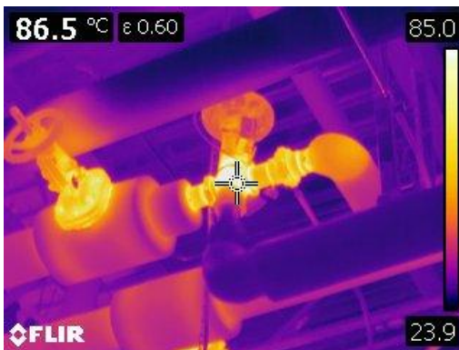
Figure 49 Thermographic image of bare three way valve and bare valve bonnet at 86° C or 186° F
