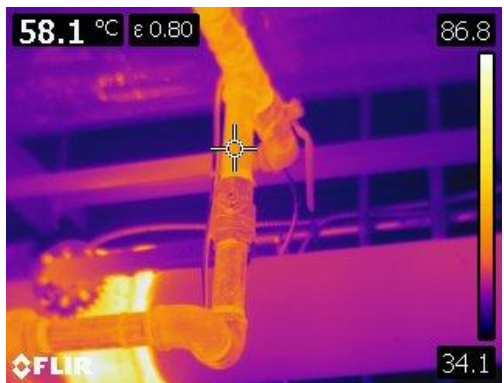
Figure 17 Thermographic image of the same 1 inch line at the other end.
