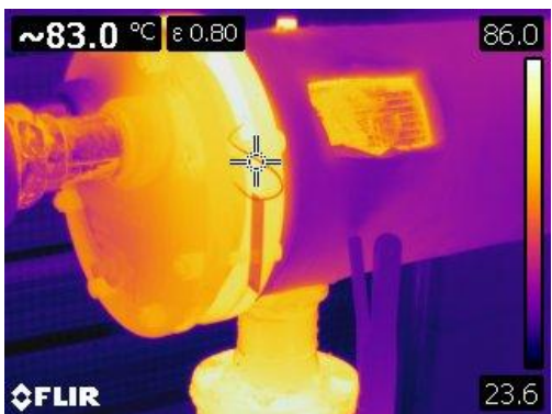
Figure 7 This is a thermographic image of the bare end of a heat exchanger.
