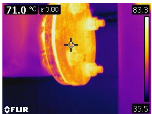
Figure 19 Thermographic image of a bare flange/endcap.
