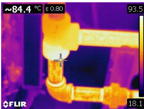
Figure 5 This Thermographic image of supply lines to a heat recovery coils.
