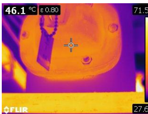
Figure 13 This thermographic image is of a bare valve bonnet.
