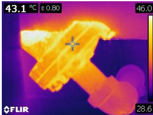
Figure 11 This thermographic image is of bare drain from the heat exchanger.
