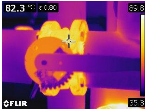
Figure 21 Thermographic image of a bare gate valve.
