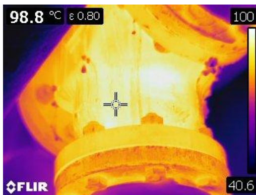
Figure 25 Thermographic image of a large bore three way valve.
