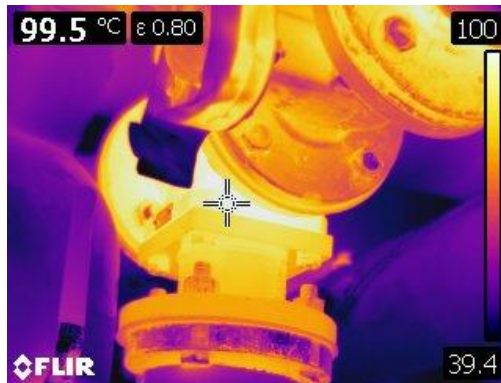
Figure 23 Thermographic image of a three way mixing valve and a gate valve.
