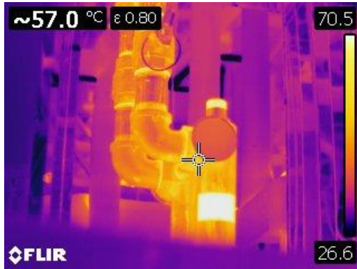
Figure 3 This thermographic image of copper piping within a stainless cabinet.
