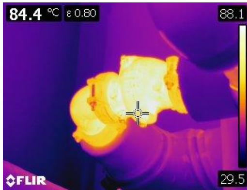
Figure 19 Thermographic image of a bare Victaulic elbow and backflow preventer.
