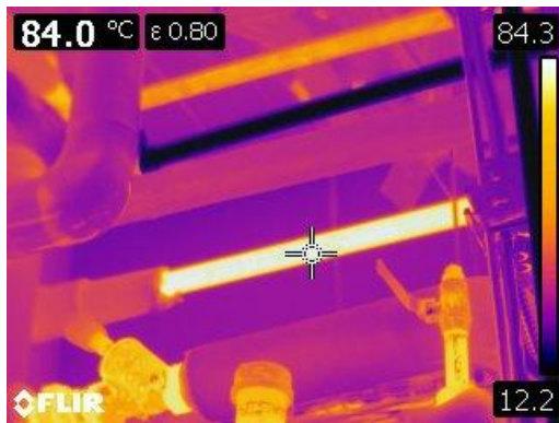
Figure 7 This is a thermographic image of a bare 1 1/4 pipe above the boilers.
