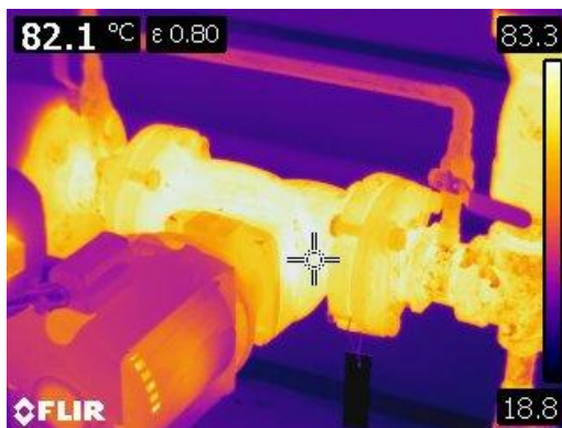
Figure 23 Thermographic image of motorized pump on heating system.
