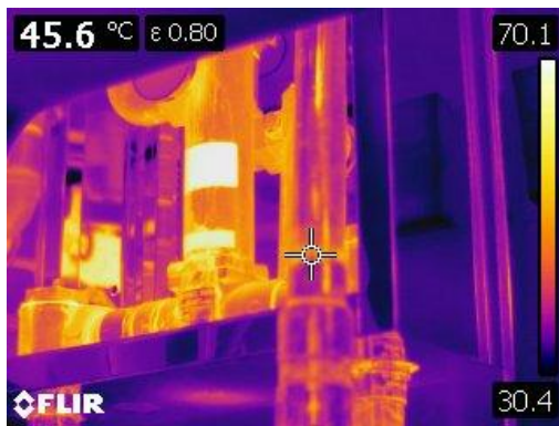
Figure 5 This Thermographic image of the copper piping within the cabinet and leaving the cabinet.
