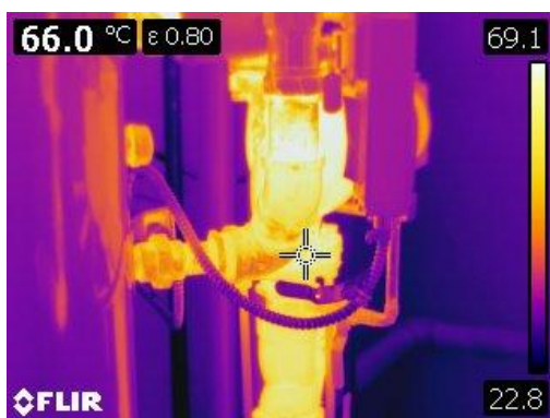
Figure 17 Thermographic image of a bare circulation pump and piping.
