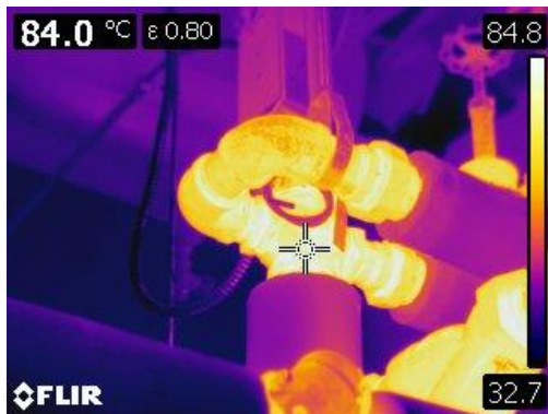
Figure 11 This thermographic image is of bare 1 1/4 iron pipe and associated fittings and valves.
