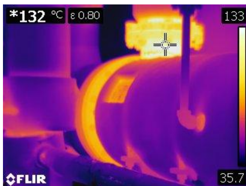
Figure 97 Thermographic image of heat exchanger flange at 132° C or 269° F
