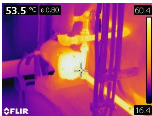
Figure 113 Thermographic image of a motorized pump and piping at 53.5° C or 128° F
