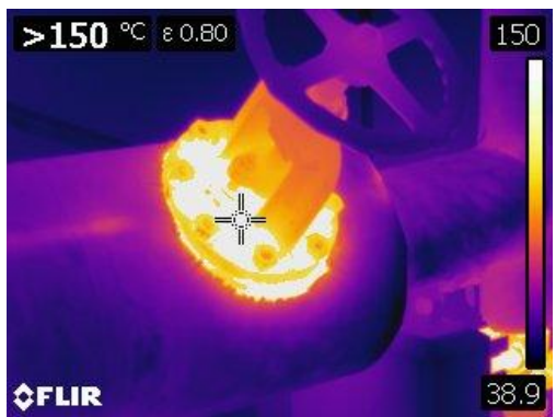
Figure 91 Thermographic image of bare valve bonnet on steam line at 150° C or 302° F
