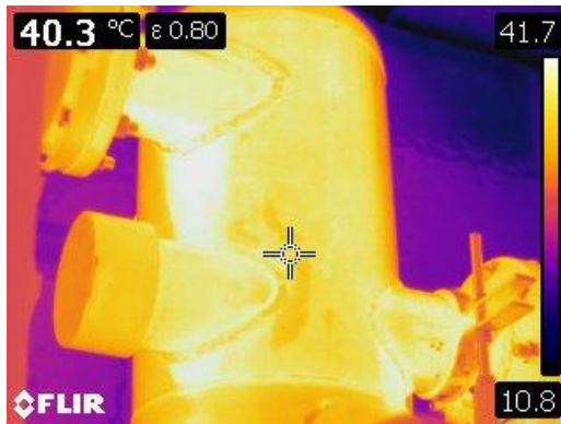
Figure 25 Thermographic image of a receiver tank above heat exchanger at 40.3° C or 106° F.
