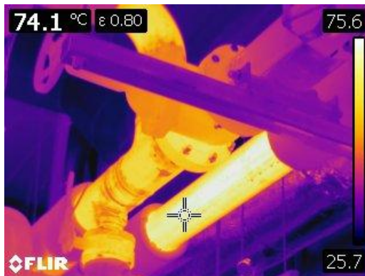
Figure 67 Thermographic image of bare pipe and flanges at 74° C or 165° F
