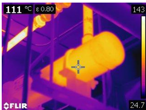
Figure 109 Thermographic image of a small heat exchanger at 111° C or 231° F
