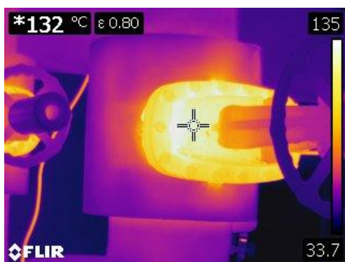
Figure 47 Thermographic image of bare vane bonnets at 132° C or 269° F.
