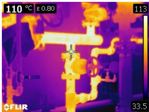
Figure 3 This thermographic image of exposed pumps and pipe at 111° C or 230° F.
