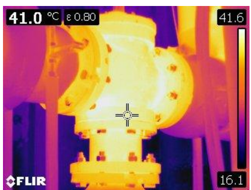
Figure 21 Thermographic image of the heat exchanger head at 41.4° C or 106° F.
