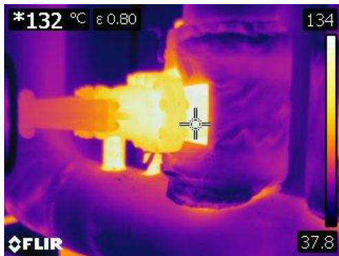
Figure 15 This thermographic image is of bare valve bonnets at 132° C or 269° F
