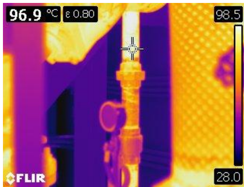
Figure 45 Thermographic image of bare stainless flex hoses from pumps at 96.9° C or 206° F.
