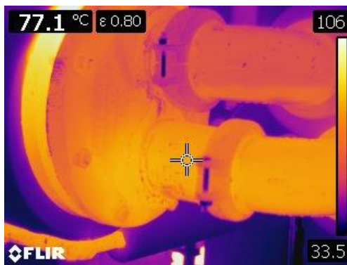
Figure 101 Thermographic image of heat exchanger head and piping at 77.1° C or 170° F
