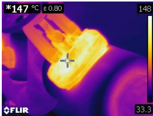
Figure 93 Thermographic image of bare valve bonnet on steam line at 147° C or 296° F
