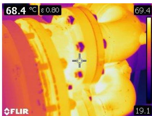
Figure 75 Thermographic image of a heat exchanger at 68.4° C or 155° F
