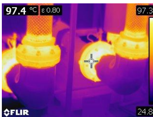
Figure 35 Thermographic image of bare pumps and flanges at 97.4° C or 207° F.
