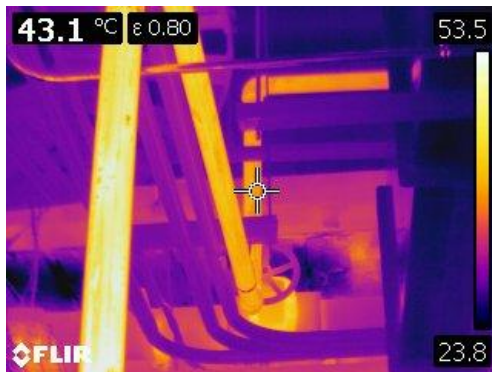
Figure 79 Thermographic image of a bare steel 2 inch line at 43.1° C or 109° F
