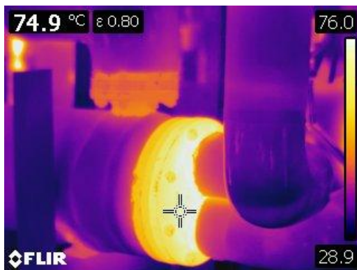
Figure 69 Thermographic image of a heat exchanger at 74.9° C or 165° F
