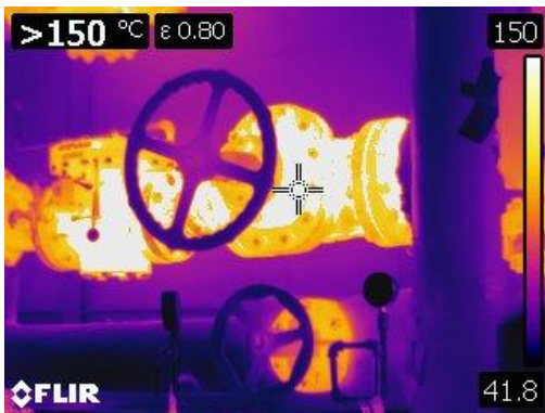
Figure 51 Thermographic image of bare valves at 150° C or 302° F
