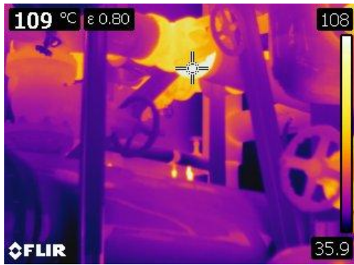
Figure 43 Thermographic image of bare valves above heat exchanger at 109° C or 228° F.
