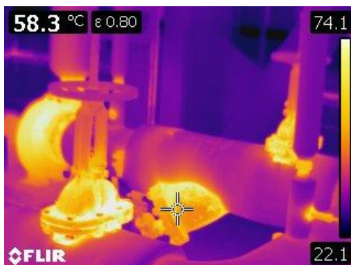
Figure 63 Thermographic image of bare valves bonnets and strainers at 58° C or 136° F
