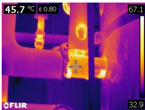
Figure 85 Thermographic image of missing insulation at hot water tanks at 45.7° C or 114° F
