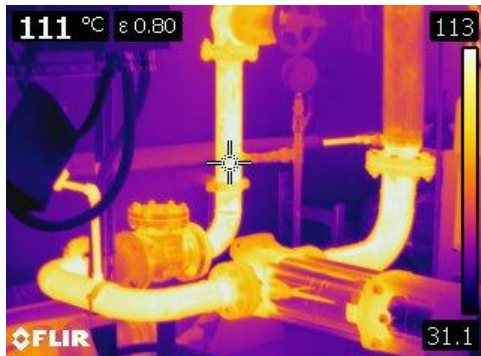
Figure 3 This thermographic image of exposed pumps and pipe at 111° C or 230° F.
