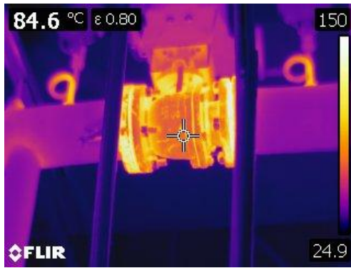
Figure 77 Thermographic image of a bare valve at 84.6° C or 184° F
