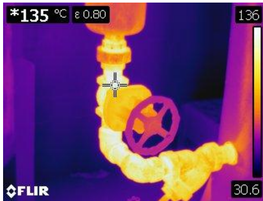
Figure 129 Thermographic image of an vertical heat exchanger piping at 135° C or 275° F
