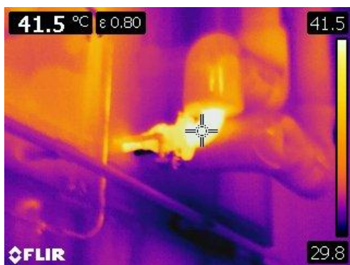
Figure 17 Thermographic image of unfinished elbows and fittings on new unit at 41.5° C or 106° F
