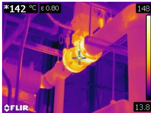
Figure 73 Thermographic image of a motorized valve at 142° C or 287° F
