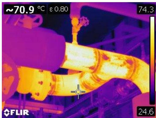
Figure 61 Thermographic image of bare 6 inch heating supply pipe at 70.9° C or 159° F
