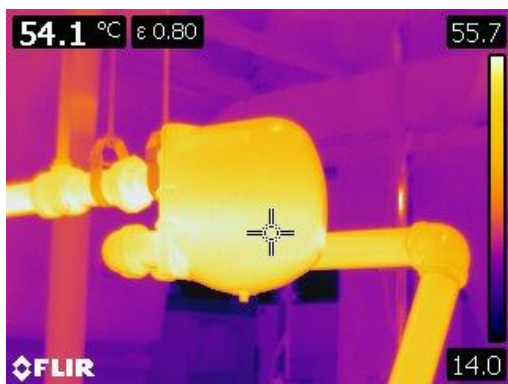
Figure 115 Thermographic image of a steam trap at 54° C or 129° F
