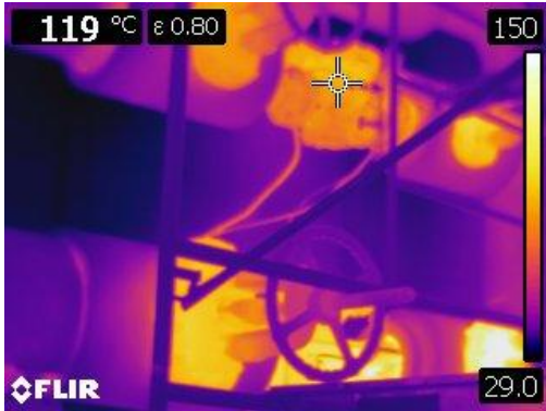
Figure 49 Thermographic image of bare valve bonnets and a pressure reducing valve at 119° C or 246° F
