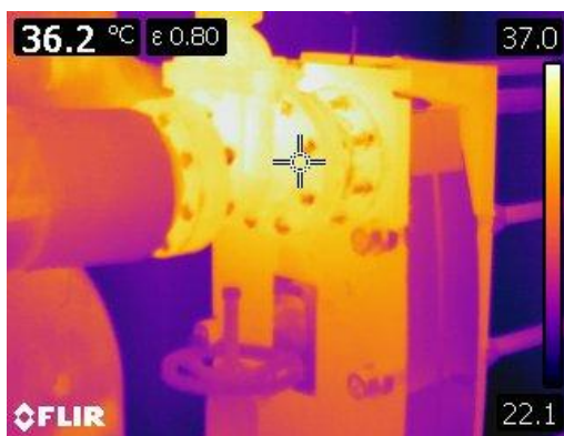
Figure 121 Thermographic image of a heat exchanger and valves at 36.2° C or 97° F
