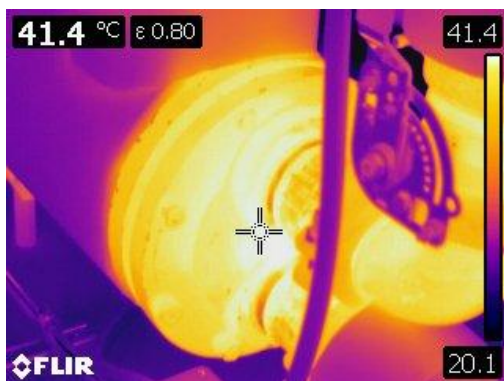
Figure 21 Thermographic image of the heat exchanger head at 41.4° C or 106° F.
