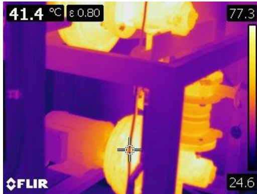
Figure 65 Thermographic image of bare motorized heating pump and piping at 41° C or 105° F
