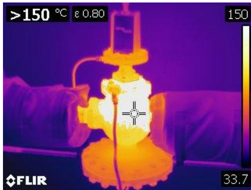
Figure 105 Thermographic image of pressure reducing valve at 150° C or 302° F
