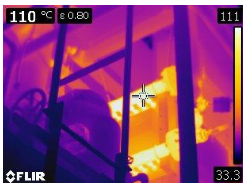
Figure 33 Thermographic image of bare piping at top of boiler at 110° C or 230° F.
