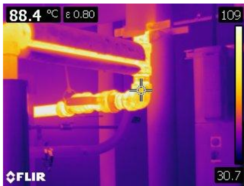
Figure 7 This is a thermographic image of a bare piping and valve at 88.4° C or 191° F.
