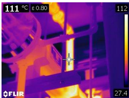
Figure 111 Thermographic image of a small heat exchanger at 111° C or 231° F
