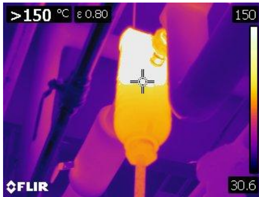
Figure 87 Thermographic image of missing insulation on steam condensate line at 150° C or 302° F
