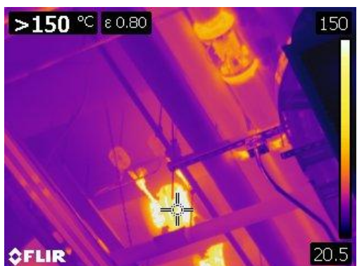
Figure 57 Thermographic image of bare flanges at 150° C or 302° F
