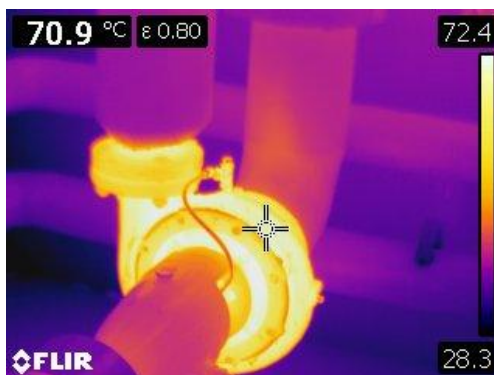
Figure 103 Thermographic image of motorized pump at 77.1° C or 170° F
