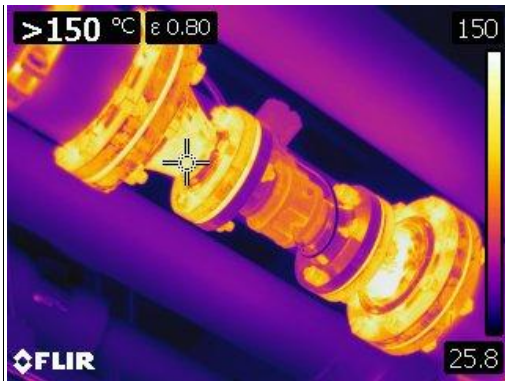
Figure 71 Thermographic image of a bare flow meter and flanges at 150° C or 302° F
