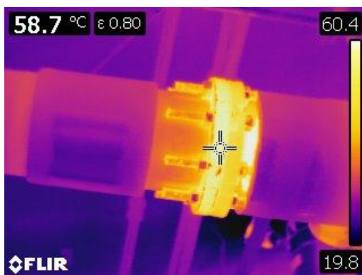
Figure 21 Thermographic image of a bare flange tying into existing systems.
