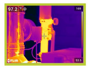
Operating Temperature, Ambient Temperature, Insulation selected 148\*F 65\*F Fiberglass Emittance of Surface
