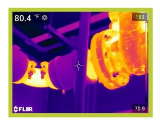
Operating Temperature, Ambient Temperature, Insulation selected 154\*F 65\*F Fiberglass Emittance of Surface0.95Expected Useful Life of Insulation System20 yrs.Operating hours per year8320Efficiency of fuel Conversion%75%
