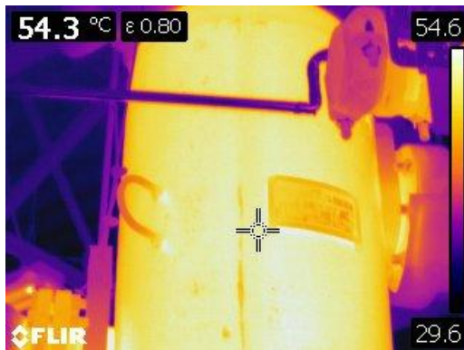
Figure 79 thermographic image of a receiver tank.
