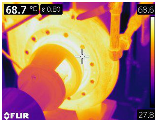
Figure 17 Thermographic image of a Personnel protection hazard at floor level
