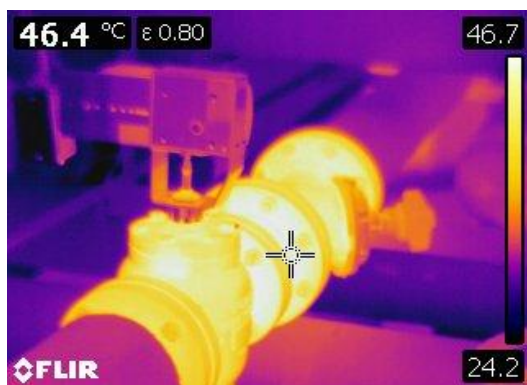
Figure 65 Thermographic image exposed motorized three way valve.
