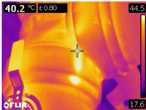
Figure 5 This Thermographic image of a Victaulic Tee which has been insulated with flex wrap. Note the high rate of heat loss as indicated by the bright color.
