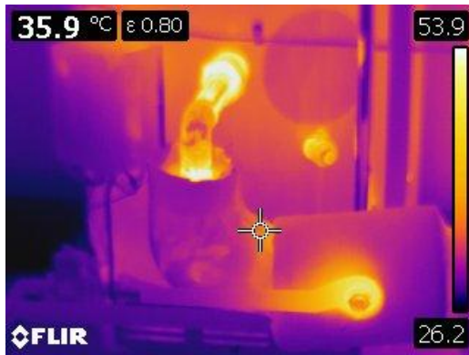
Figure 69 Thermographic image of damaged piping from hot water tank.
