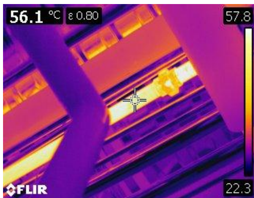
Figure 13 This thermographic image is of a bare 1.25 inch pipe 21 feet in length against the ceiling of the room.
