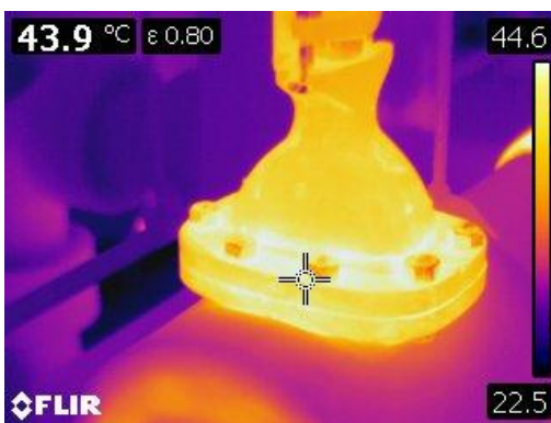
Figure 61 Thermographic image exposed valve bonnet.
