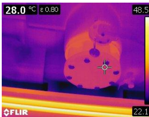
Figure 41 Thermographic image of exposed gate valves.
