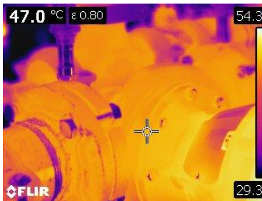
Figure 71 Thermographic image of motorized circulation pump.
