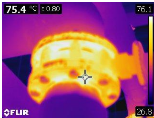
Figure 49 Thermographic image of bare gate valve operating at 75.4C or 167F.
