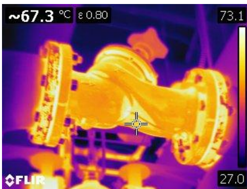
Figure 55 Thermographic image of exposed control valve.
