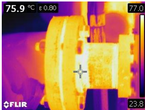
Figure 53 Thermographic image of exposed flanges at the back of the boiler
