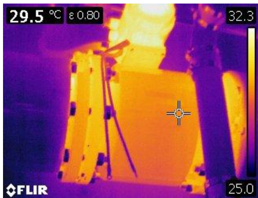
Figure 39 Thermographic image of a flow meter on the heating side.
