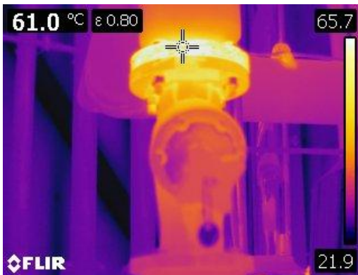
Figure 21 Thermographic image of a control valve adjacent to boiler.
