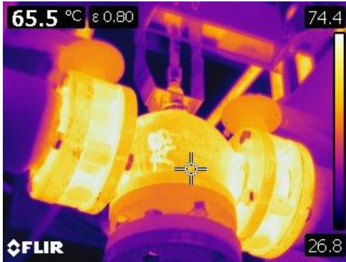
Figure 57 Thermographic image of exposed three way valve.
