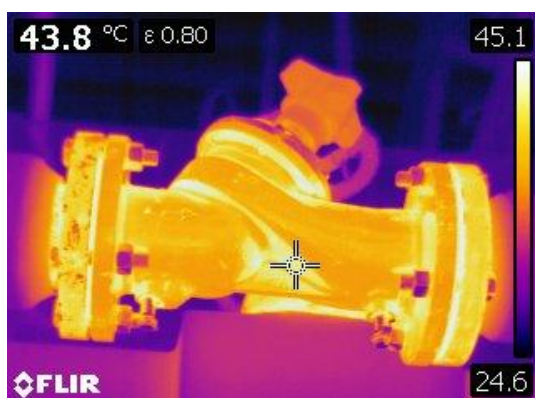
Figure 67 Thermographic image of bare control valve
