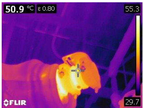
Figure 83 thermographic image of unfinished heating piping.
