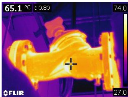
Figure 45 Thermographic image of exposed control valve.
