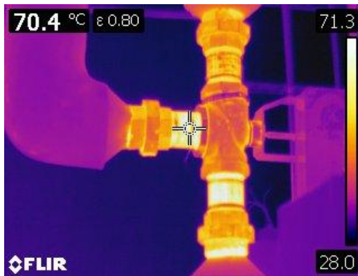
Figure 15 This thermographic image is of a bare three way valve operating at a high temperature.
