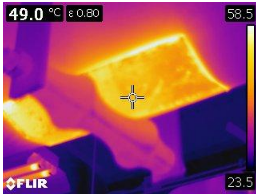
Figure 29 Thermographic image of hanger supports without insulation behind plates.
