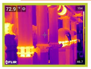
Operating Temperature, Ambient Temperature, Insulation selected 133\*F 70\*F Fiberglass Emittance of Surface
