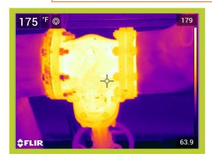
Operating Temperature, Ambient Temperature, Insulation selected 175\*F 70\*F Fiberglass Emittance of Surface
