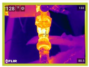
Operating Temperature, Ambient Temperature, Insulation selected 133\*F 73\*F Fiberglass Emittance of Surface
