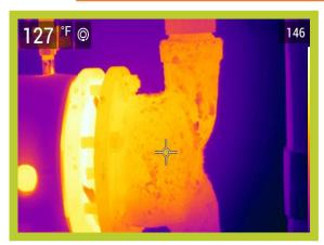
Operating Temperature, Ambient Temperature, Insulation selected 146\*F 75\*F Fiberglass Emittance of Surface Expected Useful Life of Insulation System Operating hours per year Efficiency of fuel Conversion% Selected fuel
