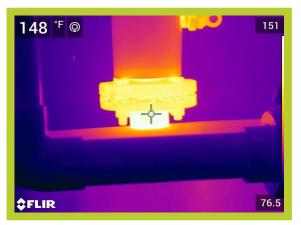
Operating Temperature, Ambient Temperature, Insulation selected 151\*F 75\*F Fiberglass Emittance of Surface
