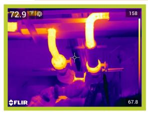
Operating Temperature, Ambient Temperature, Insulation selected 158\*F 73\*F Fiberglass Emittance of Surface Expected Useful Life of Insulation System Operating hours per year Efficiency of fuel Conversion% Selected fuel
