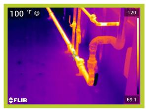
Operating Temperature, Ambient Temperature, Insulation selected 118\*F 73\*F Fiberglass Emittance of Surface
