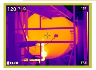
Operating Temperature, Ambient Temperature, Insulation selected 128\*F 70\*F Fiberglass Emittance of Surface
