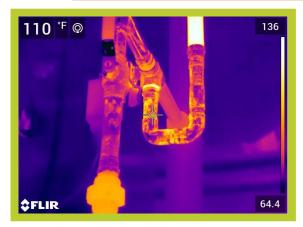
Operating Temperature, Ambient Temperature, Insulation selected 110\*F 73\*F Fiberglass Emittance of Surface
