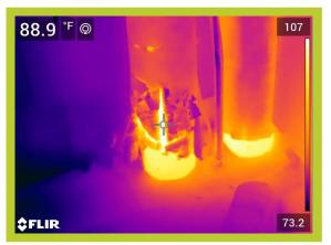
Operating Temperature, Ambient Temperature, Insulation selected 107\*F 73\*F Fiberglass Emittance of Surface
