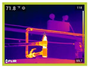
Operating Temperature, Ambient Temperature, Insulation selected 118\*F 73\*F Fiberglass Emittance of Surface Expected Useful Life of Insulation System Operating hours per year Efficiency of fuel Conversion% Selected fuel
