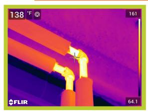
Operating Temperature, Ambient Temperature, Insulation selected 138\*F 70\*F Fiberglass Emittance of Surface
