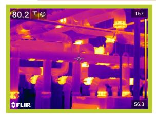
Operating Temperature, Ambient Temperature, Insulation selected 133\*F 70\*F Fiberglass Emittance of Surface Expected Useful Life of Insulation System Operating hours per year Efficiency of fuel Conversion% Selected fuel
