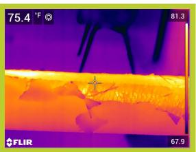
Operating Temperature, Ambient Temperature, Insulation selected 145\*F 74\*F Fiberglass Emittance of Surface
