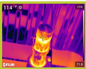
Operating Temperature, Ambient Temperature, Insulation selected 118\*F 74\*F Fiberglass Emittance of Surface
