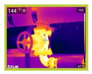
Operating Temperature, Ambient Temperature, Insulation selected 93\*F 74\*F Fiberglass Emittance of Surface0.95Expected Useful Life of Insulation System20 yrs.Operating hours per year8320Efficiency of fuel Conversion%75%
