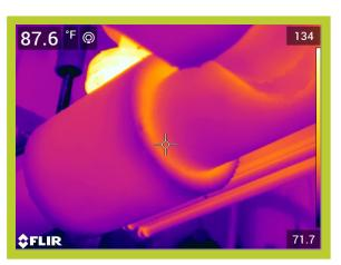
Operating Temperature, Ambient Temperature, Insulation selected 150\*F 74\*F Fiberglass Emittance of Surface0.95Expected Useful Life of Insulation System20 yrs.Operating hours per year8320Efficiency of fuel Conversion%75%
