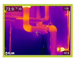
Operating Temperature, Ambient Temperature, Insulation selected 113\*F 74\*F Fiberglass Emittance of Surface
