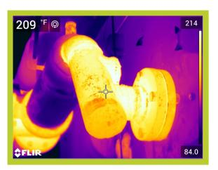
Operating Temperature, Ambient Temperature, Insulation selected 209\*F 81\*F Fiberglass
