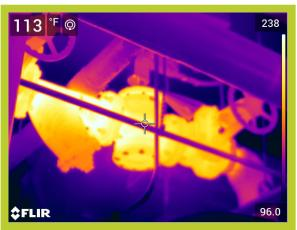
Operating Temperature, Ambient Temperature, Insulation selected 212\*F 81\*F Fiberglass Emittance of Surface
