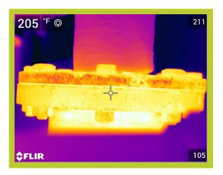
Operating Temperature, Ambient Temperature, Insulation selected 205 \*F 88\*F Fiberglass
