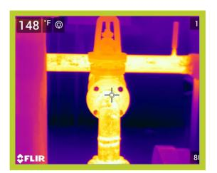
Operating Temperature, Ambient Temperature, Insulation selected 149\*F 81\*F Fiberglass
