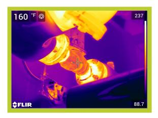
Operating Temperature, Ambient Temperature, Insulation selected 218\*F 81 \*F Fiberglass
