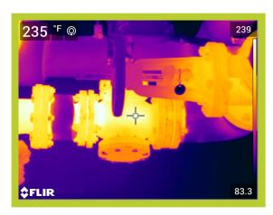
Operating Temperature, Ambient Temperature, Insulation selected 235\*F 81\*F Fiberglass
