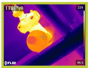
Operating Temperature, Ambient Temperature, Insulation selected 202\*F 81\*F Fiberglass
