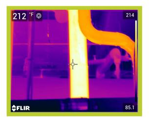
Operating Temperature, Ambient Temperature, Insulation selected 180\*F 81\*F Fiberglass Emittance of Surface0.95Expected Useful Life of Insulation System20 yrs.Operating hours per year8320Efficiency of fuel Conversion%75%
