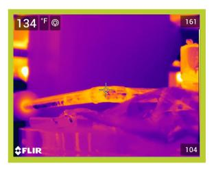
Operating Temperature, Ambient Temperature, Insulation selected 134\*F 88\*F Fiberglass
