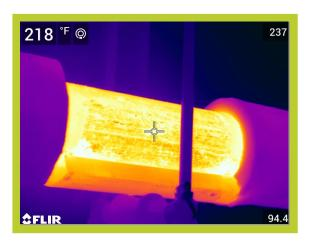
Operating Temperature, Ambient Temperature, Insulation selected 238\*F 88\*F Fiberglass
