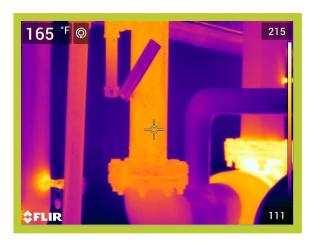
Operating Temperature, Ambient Temperature, Insulation selected 165\*F 88\*F Fiberglass
