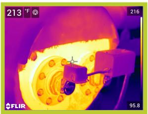
Operating Temperature, Ambient Temperature, Insulation selected 213\*F 88\*F Fiberglass
