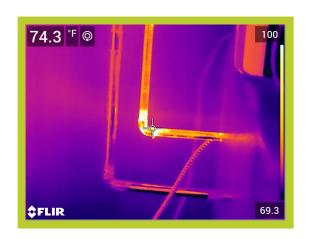
Operating Temperature, Ambient Temperature, Insulation selected 100\*F 69\*F Fiberglass Emittance of Surface
