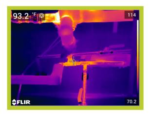
Operating Temperature, Ambient Temperature, Insulation selected 103\*F 69\*F Fiberglass Emittance of Surface
