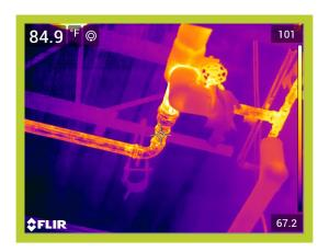
Operating Temperature, Ambient Temperature, Insulation selected 104\*F 69\*F Fiberglass Emittance of Surface Expected Useful Life of Insulation System Operating hours per year Efficiency of fuel Conversion%
