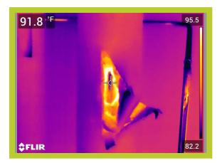
Operating Temperature, Ambient Temperature, Insulation selected 92\*F 77\*F Fiberglass Emittance of Surface Expected Useful Life of Insulation System Operating hours per year Efficiency of fuel Conversion%
