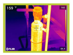
Operating Temperature, Ambient Temperature, Insulation selected 159\*F 77\*F Fiberglass Emittance of Surface0.95Expected Useful Life of Insulation System20 yrs.Operating hours per year8320Efficiency of fuel Conversion%75%
