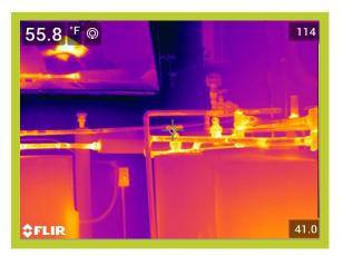
Operating Temperature, Ambient Temperature, Insulation selected 111\*F 70\*F Fiberglass Emittance of Surface Expected Useful Life of Insulation System Operating hours per year Efficiency of fuel Conversion% 0.95 20 yrs. 8760 85%
