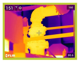
Operating Temperature, Ambient Temperature, Insulation selected 143\*F 70\*F Fiberglass Emittance of Surface
