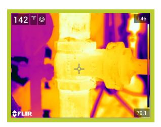
Operating Temperature, Ambient Temperature, Insulation selected 135\*F 70\*F Fiberglass
