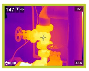
Operating Temperature, Ambient Temperature, Insulation selected 145 \*F 79 \*F Fiberglass Emittance of Surface0.95Expected Useful Life of Insulation System20 yrs.Operating hours per year8320Efficiency of fuel Conversion%75%
