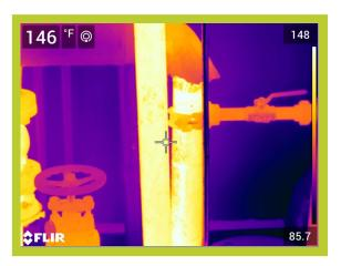
Operating Temperature, Ambient Temperature, Insulation selected 148 \*F 80 \*F Fiberglass Emittance of Surface
