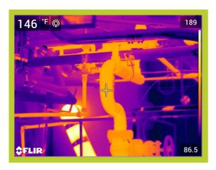
Operating Temperature, Ambient Temperature, Insulation selected 152 \*F 81\*F Fiberglass Emittance of Surface
