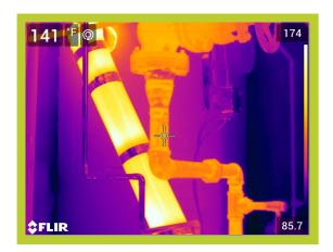
Operating Temperature, Ambient Temperature, Insulation selected 140\*F 80\*F Fiberglass Emittance of Surface Expected Useful Life of Insulation System Operating hours per year Efficiency of fuel Conversion%
