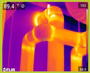
Operating Temperature, Ambient Temperature, Insulation selected 100 \*F 68 \*F Fiberglass Emittance of Surface Expected Useful Life of Insulation System Operating hours per year Efficiency of fuel Conversion% 0.95 20 yrs. 8320 75%
