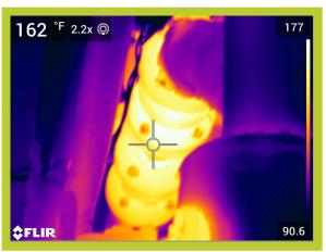
Operating Temperature, Ambient Temperature, Insulation selected 225\*F 81\*F Fiberglass Emittance of Surface
