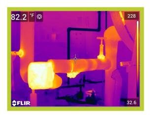
Operating Temperature, Ambient Temperature, Insulation selected 180\*F 81 \*F Fiberglass Emittance of Surface0.95Expected Useful Life of Insulation System20 yrs.Operating hours per year8320Efficiency of fuel Conversion%75%
