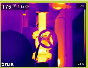
Operating Temperature, Ambient Temperature, Insulation selected 175\*F 81\*F Fiberglass Emittance of Surface Expected Useful Life of Insulation System Operating hours per year Efficiency of fuel Conversion%
