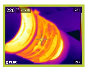
Operating Temperature, Ambient Temperature, Insulation selected 224\*F 81\*F Fiberglass Emittance of Surface
