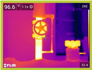
Operating Temperature, Ambient Temperature, Insulation selected 170\*F 74\*F Fiberglass Emittance of Surface 0.95
