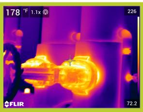
Operating Temperature, Ambient Temperature, Insulation selected 230\*F 74\*F Fiberglass Emittance of Surface0.95Expected Useful Life of Insulation System20 yrs.Operating hours per year8320Efficiency of fuel Conversion%75%
