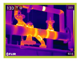
Operating Temperature, Ambient Temperature, Insulation selected 235\*F 81 \*F Fiberglass Emittance of Surface Expected Useful Life of Insulation System Operating hours per year Efficiency of fuel Conversion%
