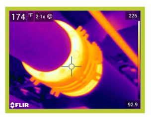
Operating Temperature, Ambient Temperature, Insulation selected 160\*F 81\*F Fiberglass Emittance of Surface
