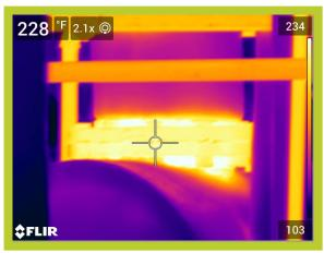
Operating Temperature, Ambient Temperature, Insulation selected 171\*F 81\*F Fiberglass Emittance of Surface
