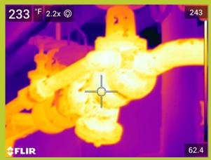
Operating Temperature, Ambient Temperature, Insulation selected 225\*F 81\*F Fiberglass Emittance of Surface Expected Useful Life of Insulation System Operating hours per year Efficiency of fuel Conversion%
