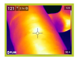
Operating Temperature, Ambient Temperature, Insulation selected 112\*F 81\*F Fiberglass Emittance of Surface
