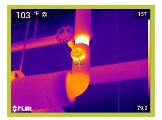
Operating Temperature, Ambient Temperature, Insulation selected 162\*F 62\*F Fiberglass
